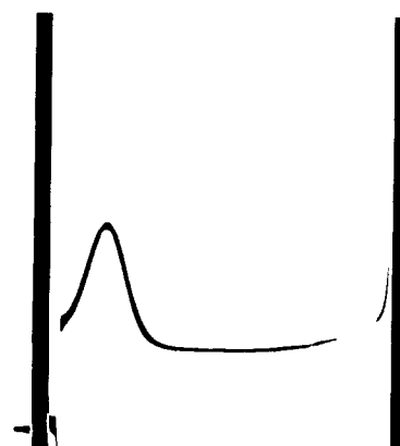
FIG. 8.—Sedimentation pattern of fraction II (1.1% protein) in 0.1 M potassium phosphate buffer, pH 8.0. Sedimentation for 60 minutes at 59,780 rpm, bar angle 60°.
